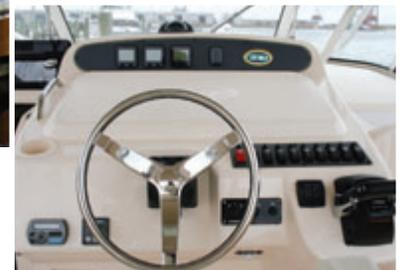
Helm console with electromechanically operated lockable electronics enclosure
