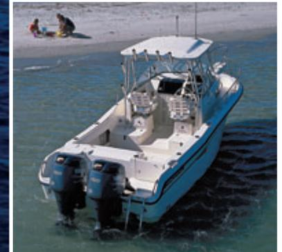
Cockpit forward showing transom door and integrated swim platform with ladder
