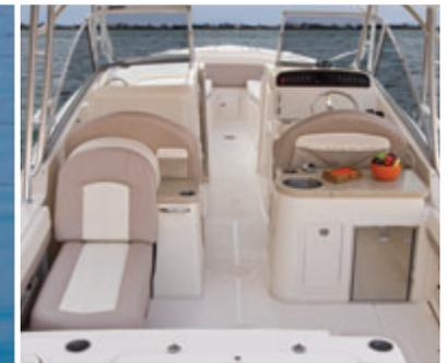
Cockpit forward area with electric extendable lounge seating. The standard wet bar includes a sink and fiberglass storage bin under the Corian® top.
