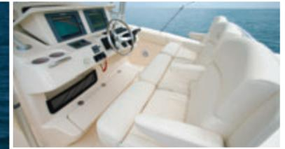
Center helm lean bar with three deluxe sliding seats with flip-up bolsters and footrest; electromechanically operated lockable electronics enclosure
