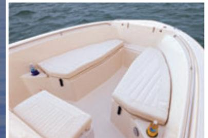
101-qt. (96 l) port and starboard forward insulated fish boxes with ob drain. Access to bow at deck level. Console forward seating with removable 72-qt. (68 l) cooler.
