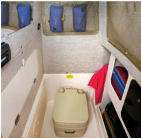
Lockable stand up console head enclosure with storage shelves and hanging locker; shown with optional portable head
