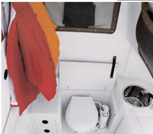
Lockable console with sink, storage and fold down cover over marine head with macerator, 10-gallon (37.9 l) holding tank and pump out
