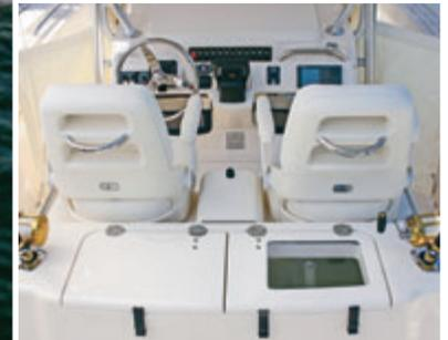
Command seating helm area with two Deluxe II adjustable sliding chairs, rigging station with freshwater sink, pullout faucet and insulated livewell
