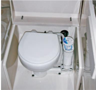
Head area in lockable cabin, with fold down cover; optional electric marine head shown
