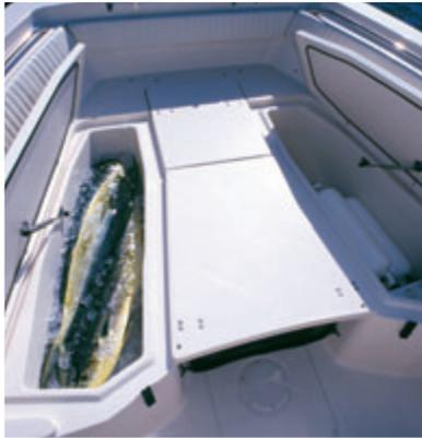
Bow insulated fish boxes with removable optional casting platform insert
