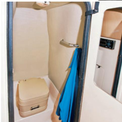
Console head area/storage compartment with dome light; optional portable head
