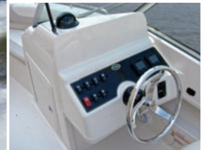
Helm station with flush mount electronics area
