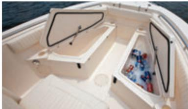
Forward port, starboard insulated boxes with cushions; optional forward bolsters
